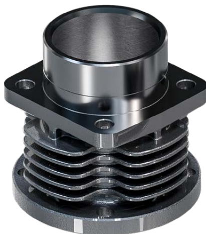
Die-cast aluminium cylinders with barrel coating in nicasil
